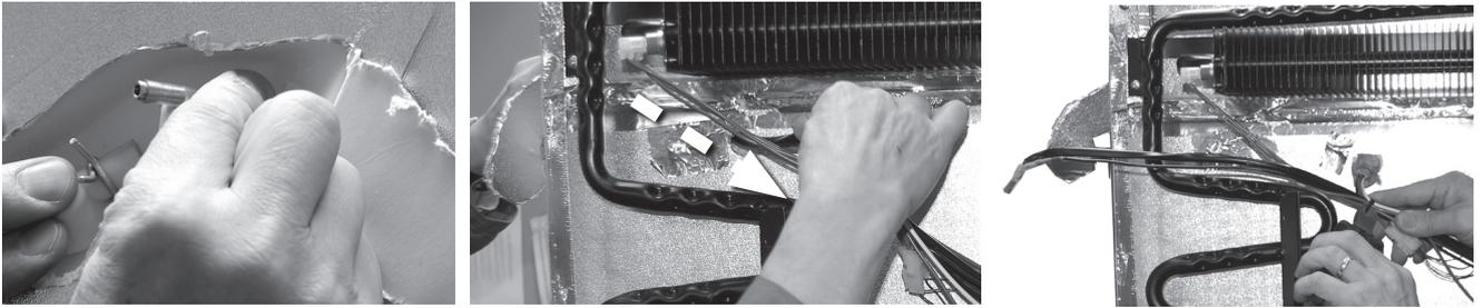
8. Loosen screws and remove the two fans. Disconnect the wires.
