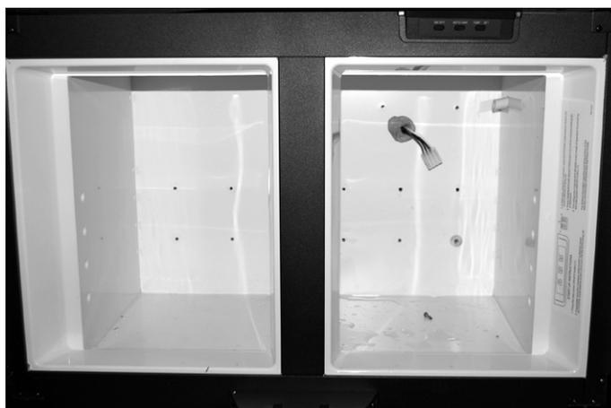
3. Open fridge doors and remove the 6 screws anchoring the evaporator fins.
