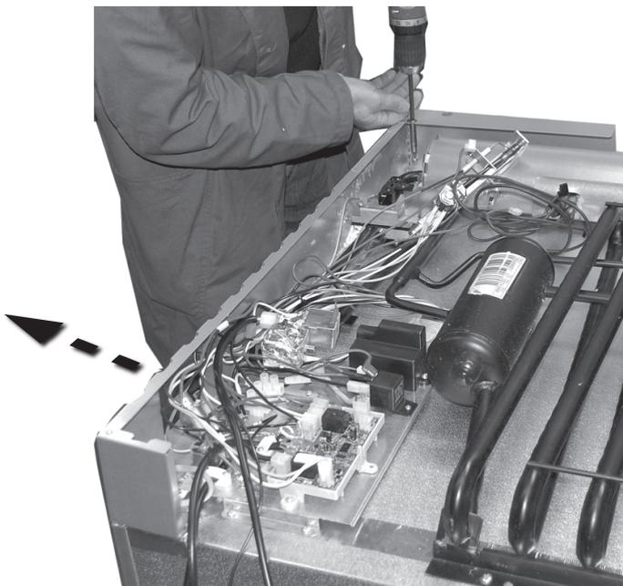
15. Loosen screw and detach grounding wire.
