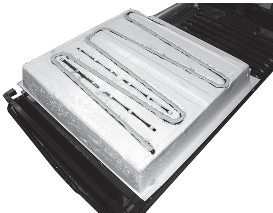
22. Place cooling unit in cabinet. Tighten the screws holding the unit to back of cabinet.
