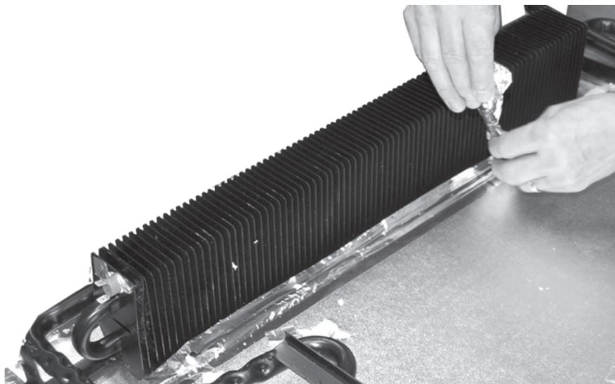
19. Insert a knife blade and cut alongside the edge.
