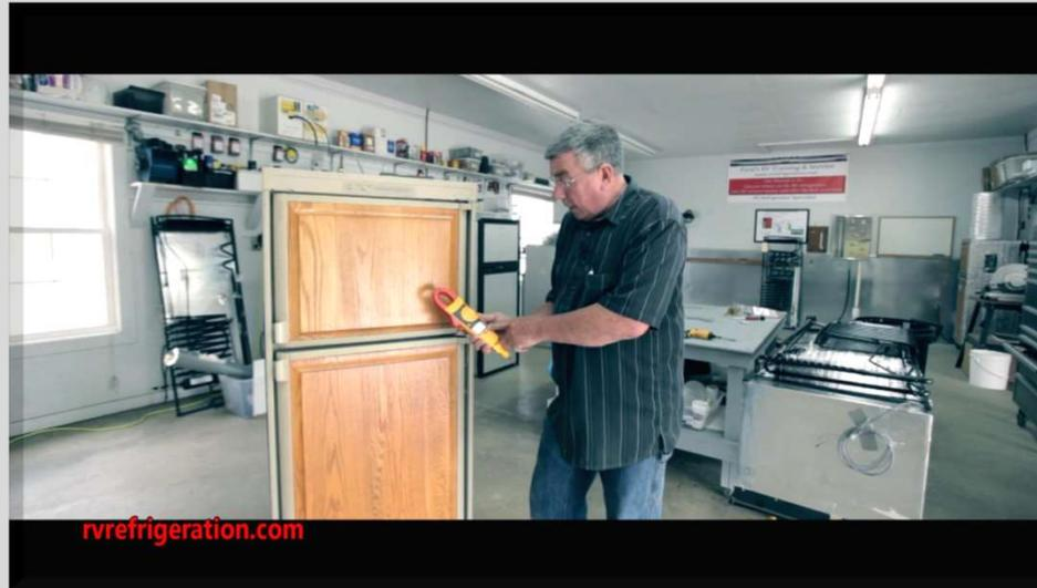
**21.1.2** Let the refrigerator operate throughout the rest of the day on LP. At the end of the day, attach the temperature probe leads to the meter and see what the Fahrenheit temperature is.
