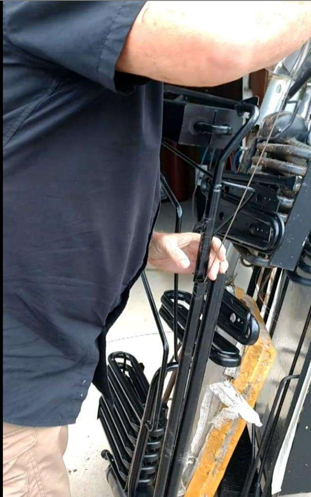
**23.2.3** Put the rod into the perc tube.
