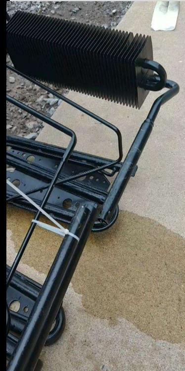
**23.3.10** Using wire ties, pull the cut sections apart and wire tie the lower section to the cooling unit so that it and the upper section are away from each other.
