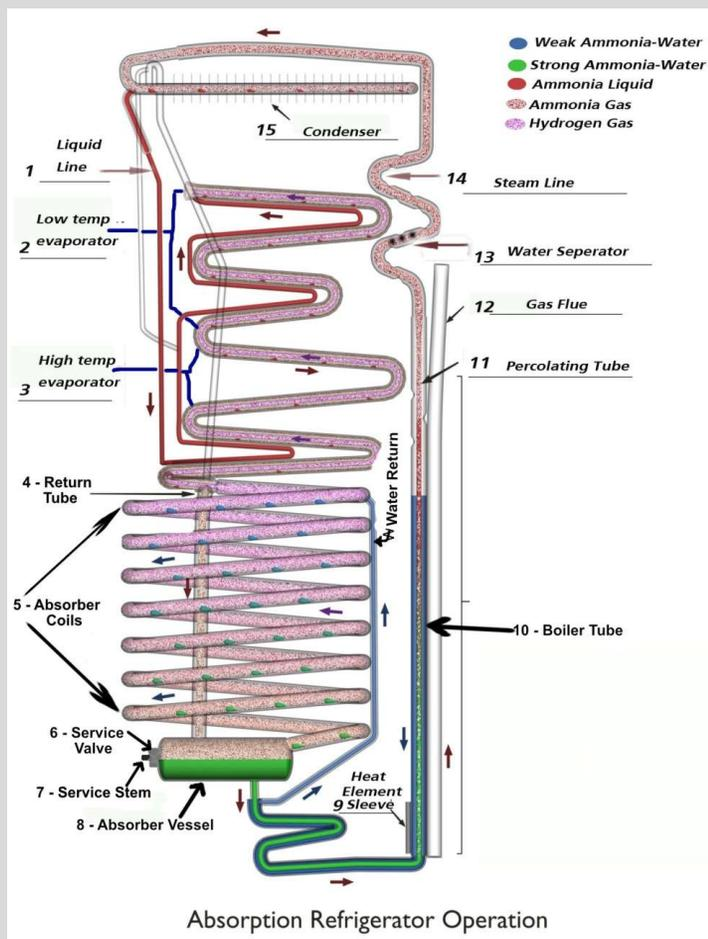
1.2.10 When the weak ammonia water drops back down the boiler tube, it is forced up to the water return where it goes back to the top of the absorber coil and flows down through the absorber coils, to the absorber vessel and is remixed with the strong ammonia water. The process starts all over again.
