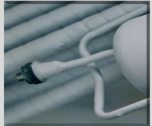
**22.2.10** Proceed to Leak Check Phase One **Procedure 9**. Be sure to leak check the service valve weld.
