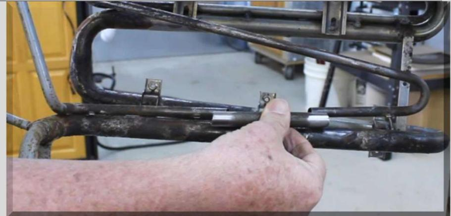
**24.1.5** Have a piece of schedule 40 seamless steel piping which is just a little larger than the liquid line to use as a coupling.
