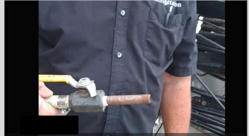
**23.3.4** On the other end of the small piece of hose, insert the 1/4" nipple that is coming out of the ball valve and secure it with a clamp.
