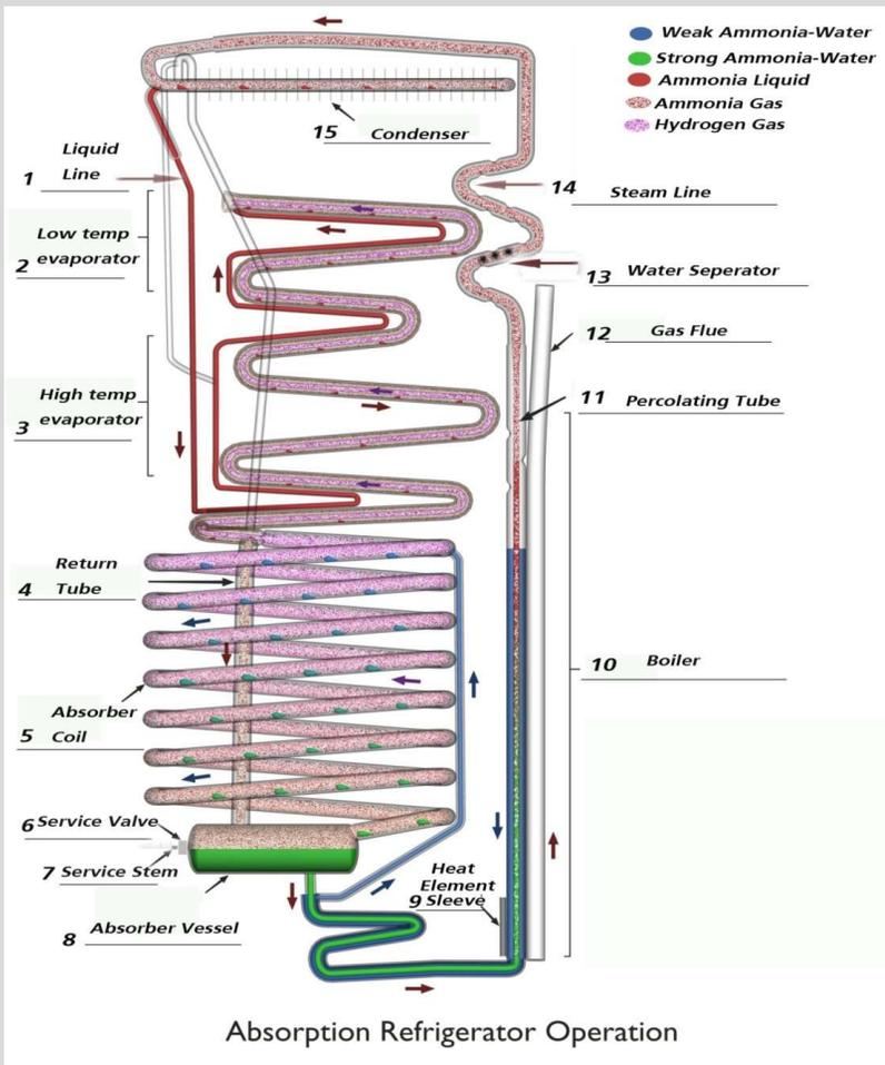
1.2.9 The **liquid saturated hydrogen** continues to fall into the return tube and down to the absorber vessel, then down to the bottom of the cooling unit where the process starts all over. When the **saturated hydrogen gas** meets the liquid in the bottom of the absorber vessel, the **hydrogen** separates and rises up through the absorber coils, then moves back up to the top of the low temp evaporator.
