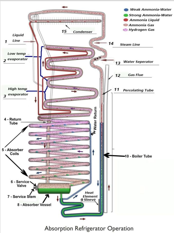
**1.2.8** Although hydrogen is the lightest gas known to man, the saturation causes it to become heavy, forcing it to fall down through the evaporator where it actually absorbs the heat out of the refrigerator, thus, absorption refrigeration.
