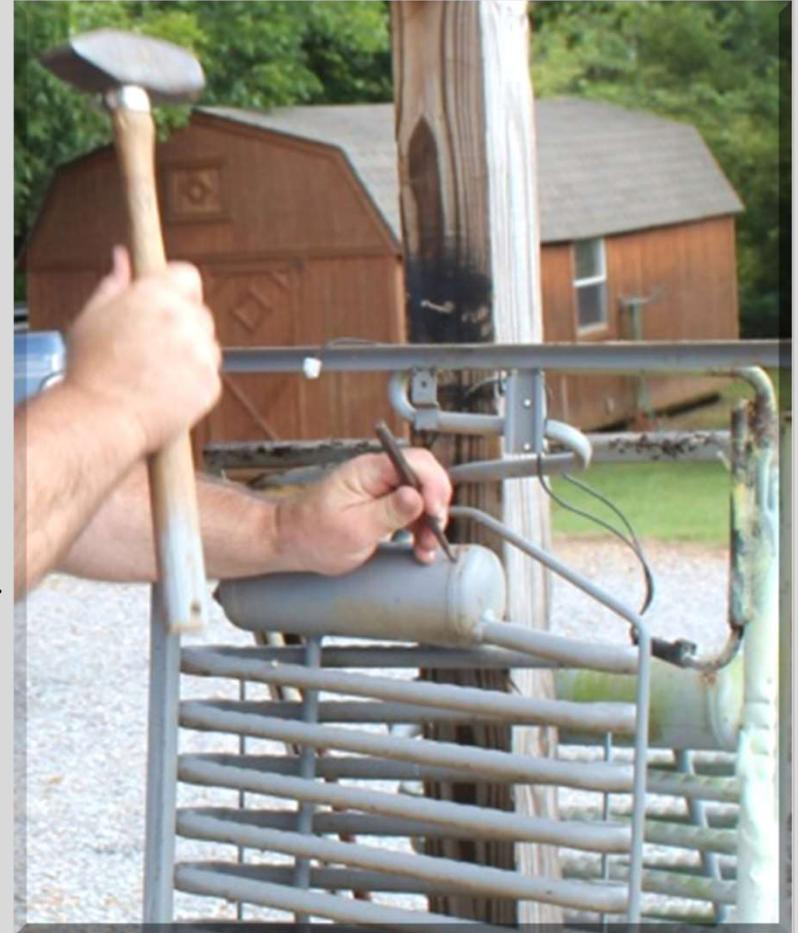
**6.1.7** After all pressure has been released, move unit to welding area. Again, stand away from the service stem.
