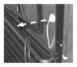
7. If applicable, detach water supply hose. Pull gently. Cut strips to disengage the hose.
