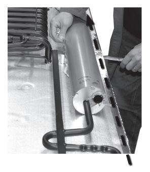
20. To remove cooling unit, take hold of the gas temperature exchanger and lift to detach.
