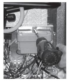
6. Gently pull to detach thermistor and then disconnect from the power module.
