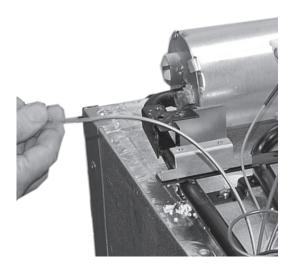
16. Loosen screws and remove bracket.
