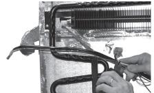
8. Loosen screws and remove the two fans. Disconnect the wires.
