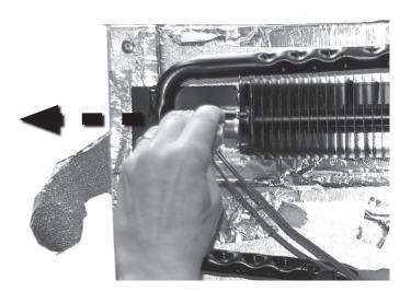
10. Loosen/open clips to disengage wires/harnesses from the back of the refrigerator. Follow these and disconnect from connection points.
