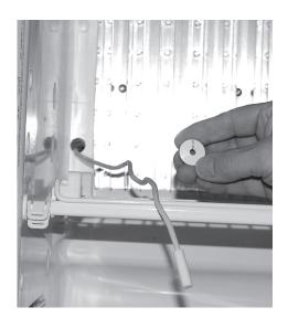
Go to the back of the refrigerator. Loosen screws and remove cover plate and power module cover.
