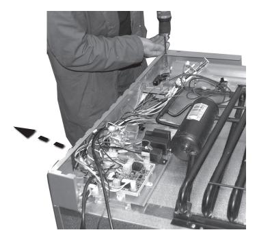
15. Loosen screw and detach grounding wire.
