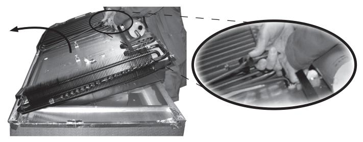
21. Locate the replacement cooling unit. Apply thermal mastic to the coils of the cooling unit.
