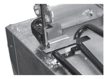
17. Remove all the screws holding the cooling unit to the refrigerator.
