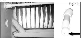
Check orifice diameter. Should be 1/4'
