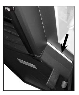
Open the freezer door and gently fold back the gasket in order to check the condition of the sealing strip. Replace or install a new sealing strip if necessary. See Figs. 2 & 2A.
