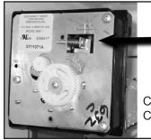
Adjusting screw for regulating the water supply
