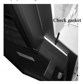
2. Open the freezer door and gently fold the gasket in order to check the condition of the sealing strip. Replace if necessary. For refrigerators lacking this strip, please install the provided sealing strip under the door gasket.
