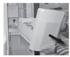
4. Remove the insulation plate by loosening the two screws. Save the screws for reinstallation.
