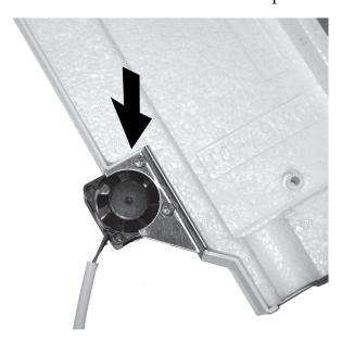
6. Reinstall the insulation plate. Fasten with the two screws removed earlier.
