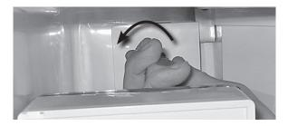
... and locate the fan connector (2-pole Molex with black/red wires). For further instructions, please see "Alternative 1". If it is *not* located here, the refrigerator is of a newer model and the connection is installed close to the fan instead. If this is the case, reinstall the cover and then, see "Alternative 2" for further instructions.
